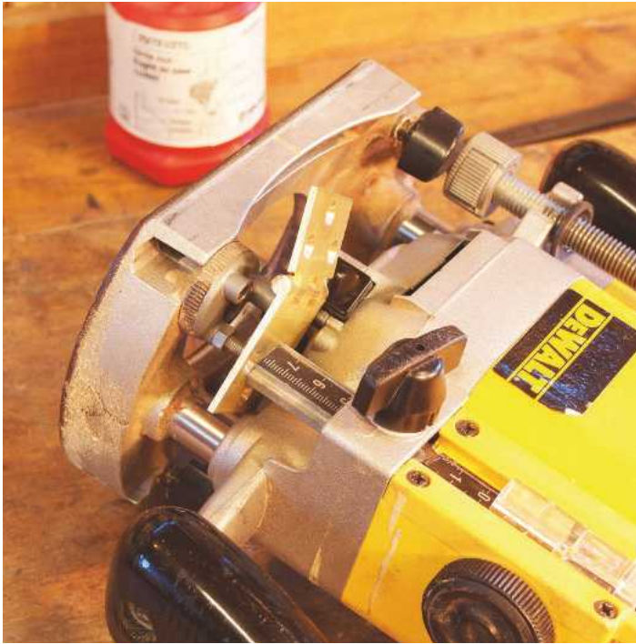
▲ Pic.11 You can set the depth using the hinge itself
